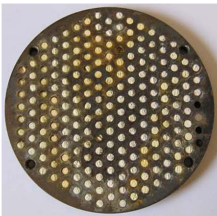
Fig. 1. Image of a stainless-steel library plate ( \varnothing 99 mm) with 207 hexagonally positioned wells ( \varnothing 3.5 mm), filled with catalysts.
